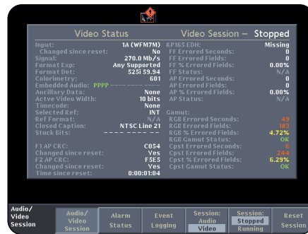
▶ WFM700 Video Session display for SMPTE 292M (HD) signal.
